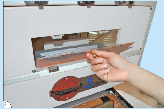
2. 自動收料於操作者前方，取料便捷 Automatic stacking in front of the operator, easy to collect the sleeve plackets
