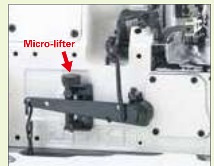
Bottom and top differential-feed micro adjustment mechanism
