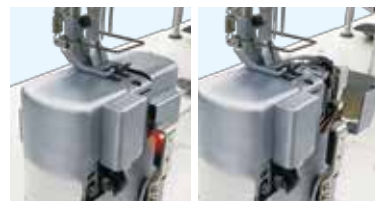
② Hook cover with an open/close sensor
